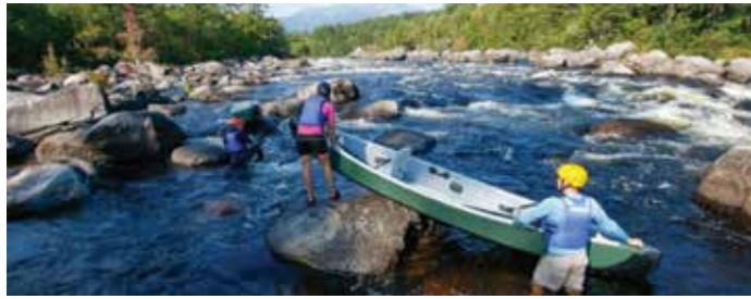
The Sea Eagle Travel Canoe 16 is described as the world's first high pressure all drop stitch rigid inflatable canoe. Pumped up by hand in under 10 minutes, it has three inflatable panels, slab sides and floor, in addition to inflatable seats. It is 4.88m long and weighs 27kg. It has plastic end fittings to aid tracking, removable skeg, front and rear spraydecks, four floor drain plugs and six securing D rings. The slab inflated panels are sufficiently rigid for the canoe to be used for gunwale bobbing.
