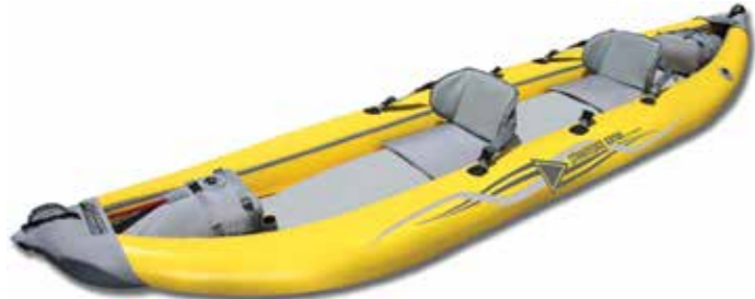
The Straightedge 2 by Advanced Elements is of more conventional inflated tube construction but has aluminium end fittings to aid tracking. It weighs 21kg and is 4m long.
